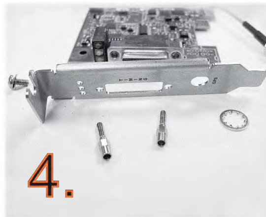
Figure 3-1: Bracket change procedure
